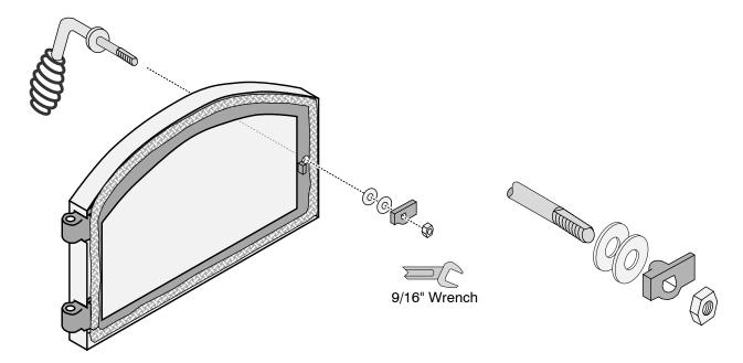
6. Replace the door on the hinges and latch the door.
