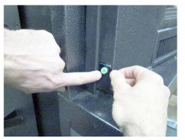
Connect the igniter assembly wires; orientation does not matter. Connect the start button wires to the igniter assembly.
