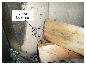
3. Place additional pieces of wood directly in front and in back of the piece of wood placed in step 2. Make sure the wood runs parallel to the igniter air flow and is spaced far enough apart to allow air to flow.
