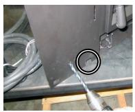
Route the igniter cord through the "mouse hole" in the left side of the panel as shown above. Attach the fa the panel.
