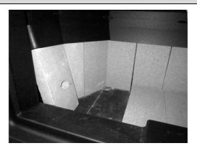
Remove the cover plate from the side of the insert as shown below. Retain the screws and gasket.
