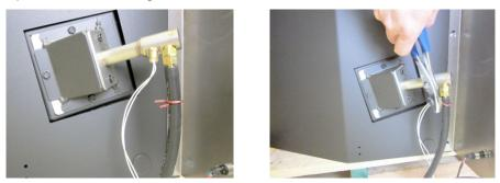
Connect the igniter wires. Orientation of the wires does not matter. Wrap the wires around the compressor hose.
