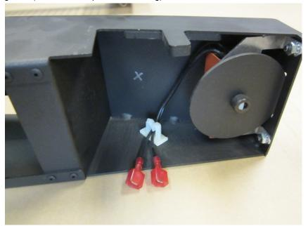
Affix the GreenStart sticker over the hole, and then insert the color-coded start button wires through the he The start button should be flush with the trim panel.
