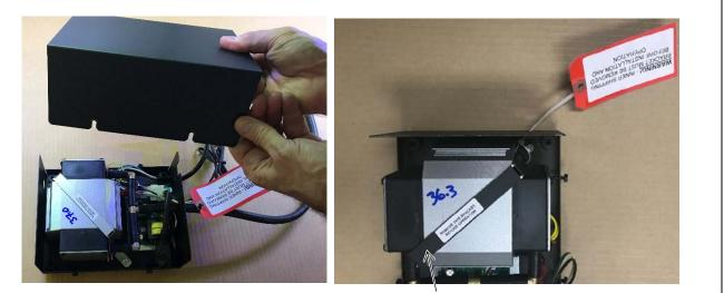
Remove the cover from the compressor assembly. Remove the shipping bracket and discard it along with the 2 screws that held it in place ( $\frac{1}{4}$ " nutdriver). Replace the cover.
