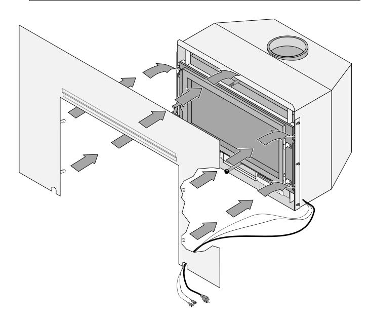
**<u>HINT</u>**: When installing the panel, route the wires through the notch on the bottom of the panel (either side).
