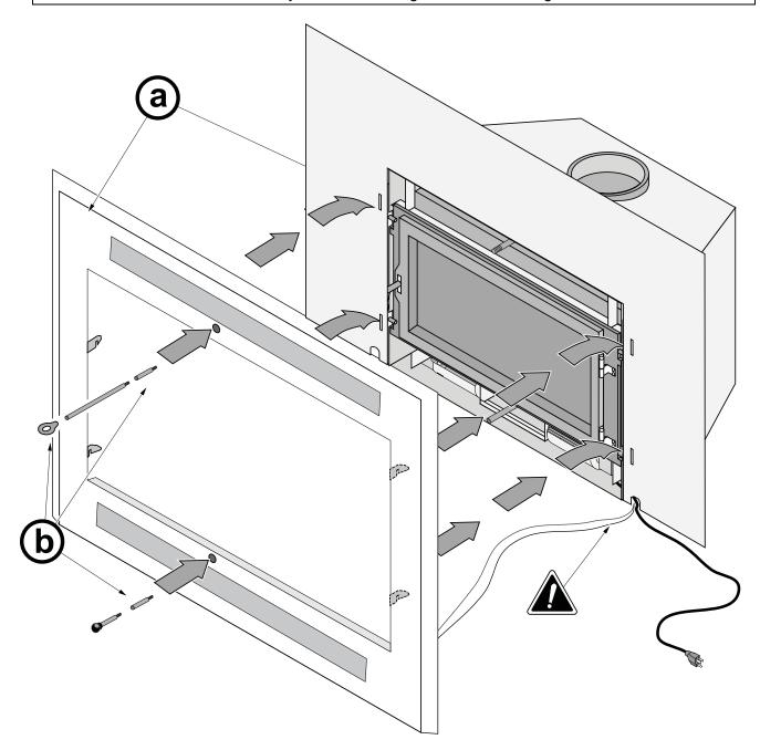
**HINT**: While installing the bypass extension, reach into the firebox and hold the bypass plate and yoke. See the manual for a detailed view.
