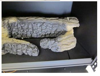
The left cross log has one hole on the bottom. Place the log so the hole fits over the left pin on the rear log. The front of the log rests on the left log (see picture for orientation).
