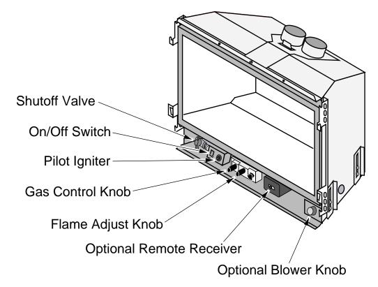
**Shutoff Valve** This valve shuts off gas to the insert.
