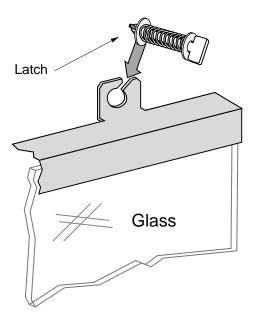
Hold the latch at an angle and insert it into the slot on the glass frame. Note how the washer fits in front of the flange on the glass frame. You will need to push slightly to get the latch to insert.
