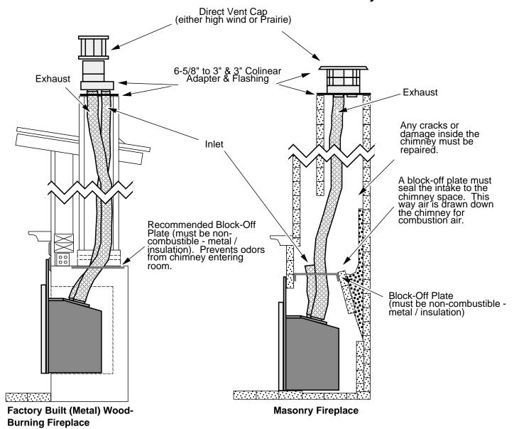
NOTE: You may use either re-line configuration with a masonry or zero-clearance fireplace.
