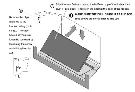
3 Install the side firebacks following the directions to the right.
