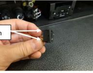
4 Guide the red and brown wires around the back of the valve and pull them out from the right side of the valve.
