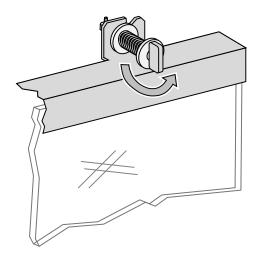
Once fully inserted, turn the latch until it is is level.
