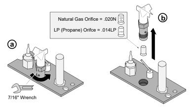
6. Remove the burner orifice and discard. Install the LP (propane) orifice.
