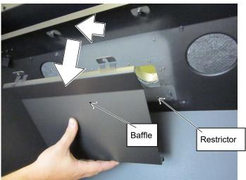
The restrictor is adjusted by loosening the two screws holding it in place. Slide the restrictor until the correct notch falls over the screws and re-tighten. Replace the baffle.
