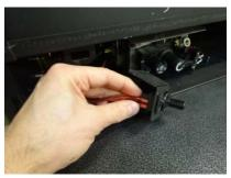
Remove the switch from the bracket and replace it with the blank that is included with the blower kit. To remove the switch squeeze the tabs on the top and bottom of the switch while pushing forward on the back side of the switch.
