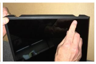
6 Place the rear fireback into position in the rear of the firebox. Hold the spacers in place on the fireback until it is in position.
