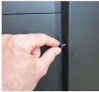
4 Replace the handle on the air restrictor.
