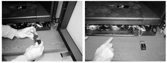
The last step is to verify the switch bracket properly contacts the micro switch on the insert: NOTE: This step is best done with the glass removed.
