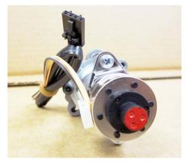
✓ Remove and Discard Both NG Manifold Covers and Orifice Gaskets – Install the LP Manifold Covers
