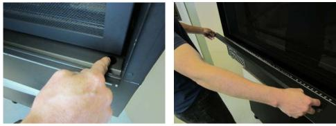
2. Remove the three screws holding the screen in place (1/4" nutdriver- magnetic driver recommended). Then pivot the screen down slightly until the clips on the bottom disengage from the glass frame.
