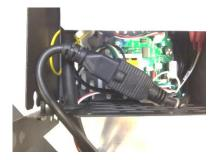
b. Route the cord through the bottom of the pump box and secure in place with the included cord restraint as shown below.
