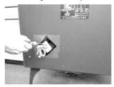
NOTE: These instructions show the compressor assembly attached to the back of the stove. Alternatively, you may place it on the floor near the stove. See the Cape Cod model installation instructions on page 12 for details.
