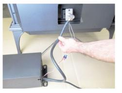
12. Attach the cover plate and igniter cover box over the igniter (cover plates are included with the stove).
