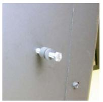
2. Tighten the bolts until the grommets contact the heat shield.
