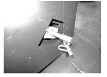
NOTE: These instructions show the compressor assembly attached to the bottom of the stove. Alternatively, you may place it on the floor near the stove. See the Cape Cod model installation instructions for details.
