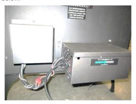
12. Plug in the compressor, then press the GreenStart start button.
