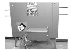
3. Tighten the bolts to secure the compressor assembly to the stove. A ratchet with an extension may help with this task.
