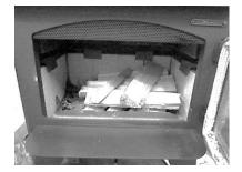
2. Make sure the air control and bypass are in the open position.
