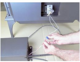
11. Attach the 1/4" tube to the nipple on the igniter.
