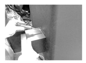
NOTE: The right side flange is tucked underneath the heat shield.
