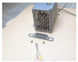
d. Install 2 grommets (both sides) into the foot plates.
