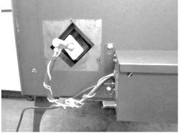
8. Attach the cover box to the heat shield as shown below, using the screws removed in step 2. If your unit does not include these holes, drill the holes with the included bit.
