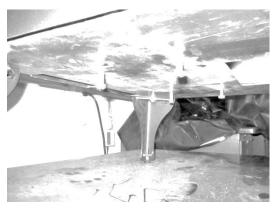
9. Place the compressor assembly under the stove with the power cord to the left (as viewed from the front of the stove).
