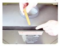
4. Remove the backing from the silicone gasket.
