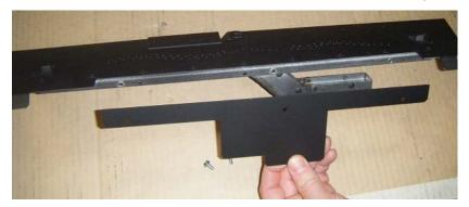
6. Replace the rear burner and secure with the attachment screw.
