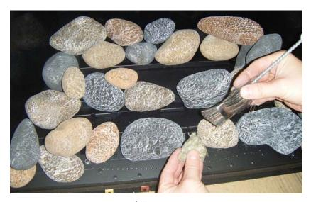
The rock wool should be approximately 1/8" thick over the burner ports.
