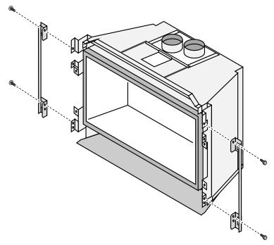
2. Bend the mounting tabs back 90° (see illustration below). Attach the surround panel as shown below.
