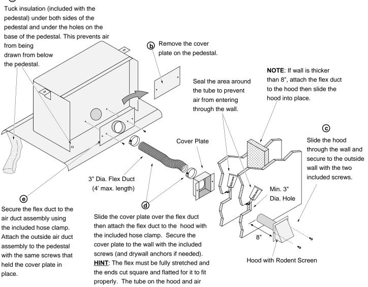
duct may be crimped if necessary.
