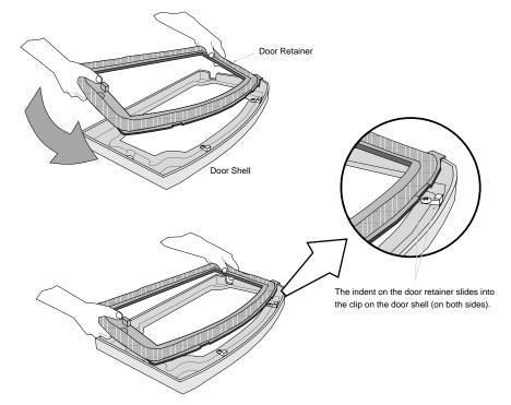
4. Remove the glass clips holding the glass in place. Remove the glass (and any remnants). The glass gasket lays between the glass and door retainer (use the existing gasket or SKU 224-11086). Place the glass in place over the gasket and replace the glass clips to secure the glass.
