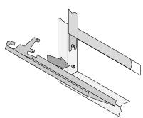
Hold the grill at an angle and insert the lower slot over the bushing on the fireplace (both sides). You may need to press on the grill to get the tab over the bushing (this prevents the grill from accidentally falling off).
