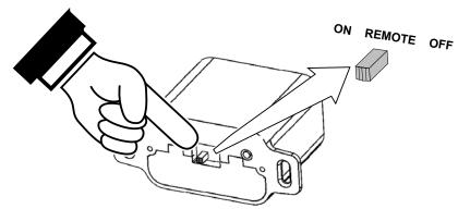
**NOTE**: When the battery holder switch is turned to ON or OFF, the mode settings (Flame Height, Comfort Control) will remain in the same state as before the switch was moved (i.e.: the IFC "remembers" the last setting). If you wish to adjust the mode settings use the transmitter mode button to adjust the settings (see "Mode Controls" on page 13). The thermostat and burner on/off operating functions will not work on the transmitter.
