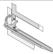
Swing the grill upwards to engage the upper slot.
