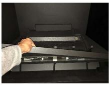
• Locate the burned out bulb and remove it from the socket by pulling the bulb directly away from socket (do not twist).
