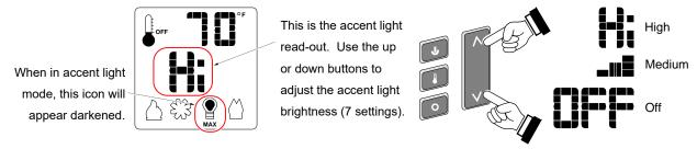
**HINT**: If you wish to leave the accent light on while turning the burner off, adjust the Flame Height to "OFF" (see above).
