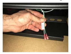
2 Connect the Green and White wires from the back of the remote to the "REMOTE" wires found in step 1.
