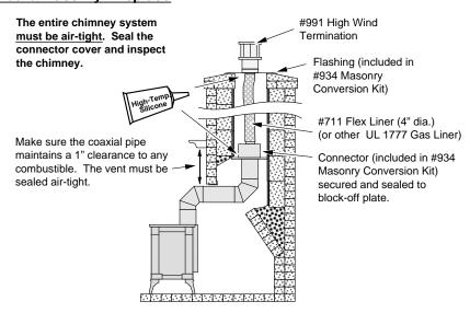
\*CAUTION: This vent configuration is not covered under the appliance safety standard (ANSI Z21.88 CSA 2.33) used in the safety certification of this appliance, however, this method has been tested by Travis Industries and it has been determined to be safe following the instructions above. Before installing the appliance using this method, contact the Authority Having Jurisdiction to determine if this installation is acceptable in your area.
