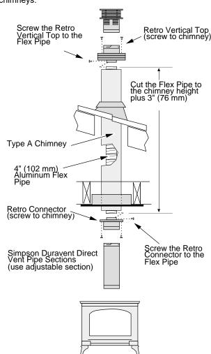
\*CAUTION: This vent configuration is not covered under the appliance safety standard (ANSI Z21.88 CSA 2.33) used in the safety certification of this appliance, however, this method has been tested by Travis Industries and it has been determined to be safe following the instructions above. Before installing the appliance using this method, contact the Authority Having Jurisdiction to determine if this installation is acceptable in your area.
