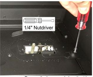
Remove the burner and place it aside.
