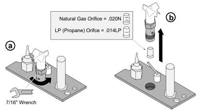
(c) Remove the burner orifice and discard. Install the LP (propane) orifice.
