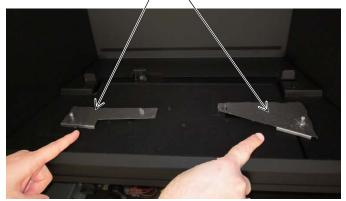
2 The rear log has two holes on the bottom. Place it over the two tabs at the back of the firebox.
