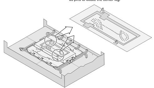
Place the center log in place. Make sure the two tabs on the log shelf insert into the two holes on the bottom of the log.
