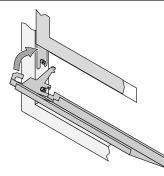
Swing the grill upwards to engage the upper slot. The grill fits inside the tabs for the barrier screen. You will need to lift the grill slightly to get it over the bushing. Once in place the grill is held in place by gravity.
