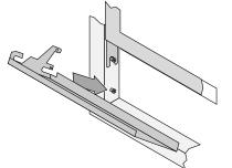
Hold the grill at an angle and insert the lower slot over the bushing on the fireplace (both sides). You may need to press on the grill to get the tab over the bushing (this prevents the grill from accidentally falling off).
