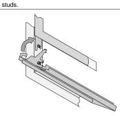
Swing the grill upwards to engage the upper slot. The grill fits inside the tabs for the barrier screen. You will need to lift the grill slightly to get it over the bushing. Once in place the grill is held in place by gravity.
