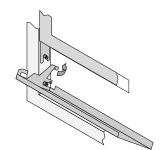
Bend the tab outward on both sides. This is the end-stop for the lower grill, it allows the grill to swing forward.
