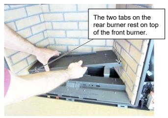
7. Re-attach the burner attachment screws (see step 1 above).
