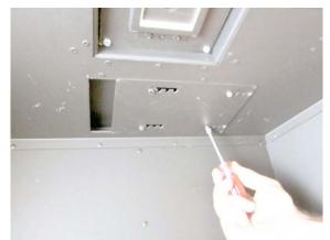
Slide the exhaust restrictor to the desired position. The photo below shows the exhaust restrictor in position #1.
