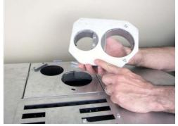
5. Attach the 4" exhaust vent to the connector and secure with at least 3 screws.
