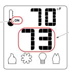
This is the target temperature on the read-out. Use the up or down buttons to adjust the target temperature.
