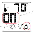
This is the comfort control read-out. Use the up button to turn on, down button to turn off (2 settings).
