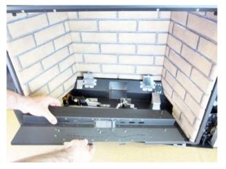
6. Replace the rear burner as shown.
