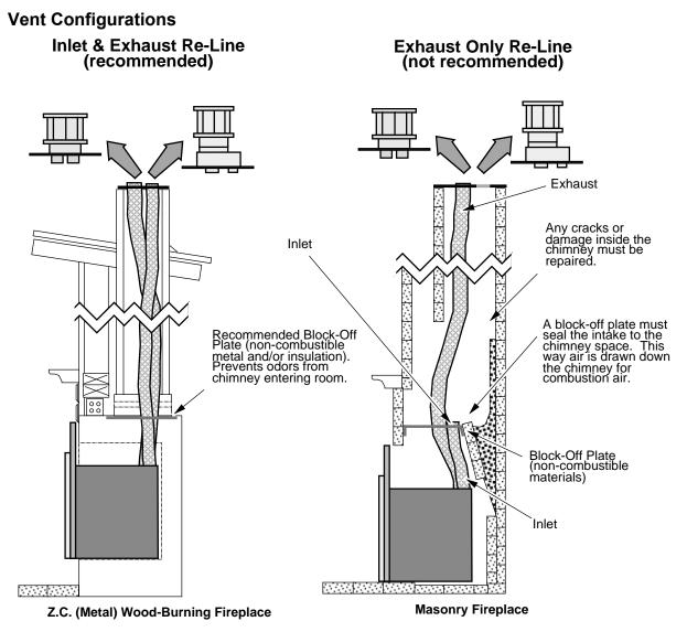
NOTE: You may use either re-line configuration with a masonry or zero-clearance fireplace.
